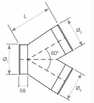
$L = \emptyset1 + 100$ ,  $\emptyset2$  and  $\emptyset3$  must be smaller than or equal to  $\emptyset1$
